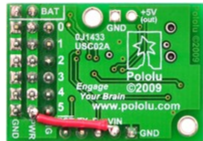
Micro Maestro configured to use a single power supply for both board and servos.
