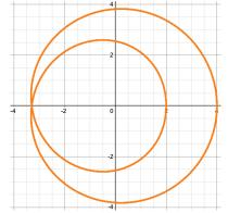
The inner circle is of radius 1. The centre of the outer wheel travels at radius 3, and then the point rolls at distance 1 around that centre.
