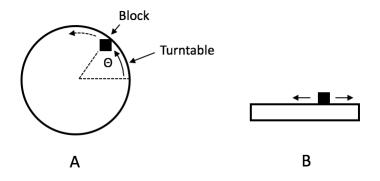
However, as seen from the side the block simply seems to move back and forth, as seen in Part B of the picture. The block's apparent position left or right of the center of the disk is proportional to  $\cos \Theta$ .
